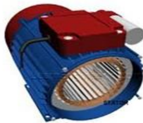
Fig. 1 The stator of an induction motor [5].
