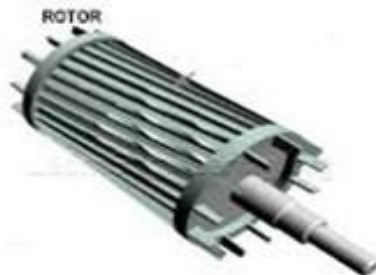
Fig. 2 The cage rotor of an induction motor [5].
