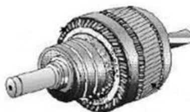
Fig. 3 The coil rotor of an induction motor [5].
